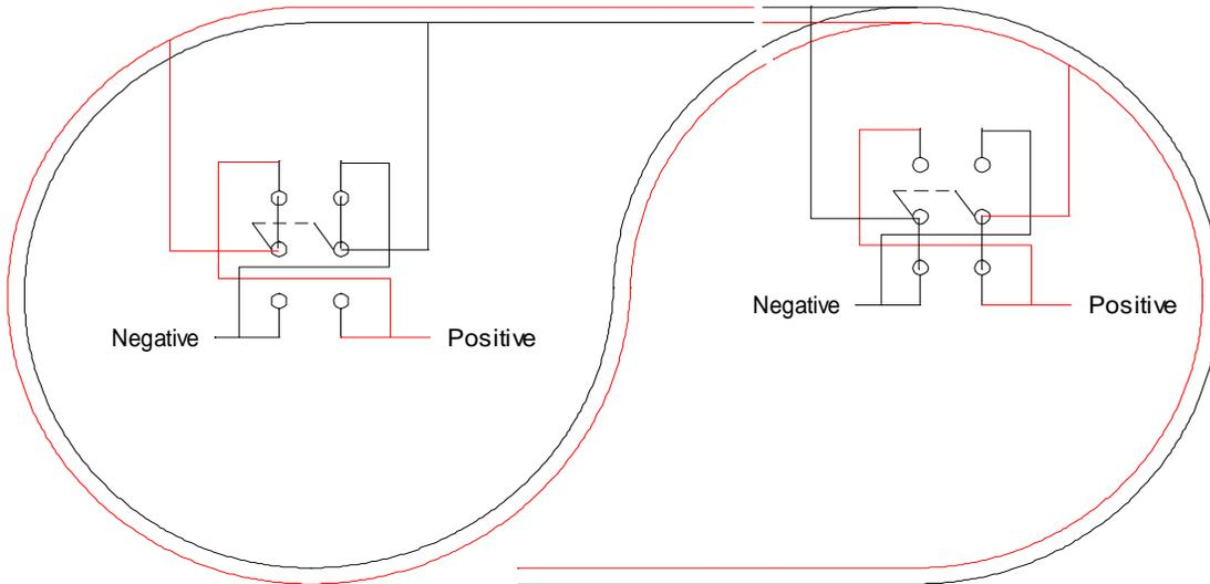
4. When a wye is used, similar controls are needed. In schematic below, the train enters from the left and turns down the leg of the wye. The polarity of the isolated section is not important as the train isn't entering that section yet.
