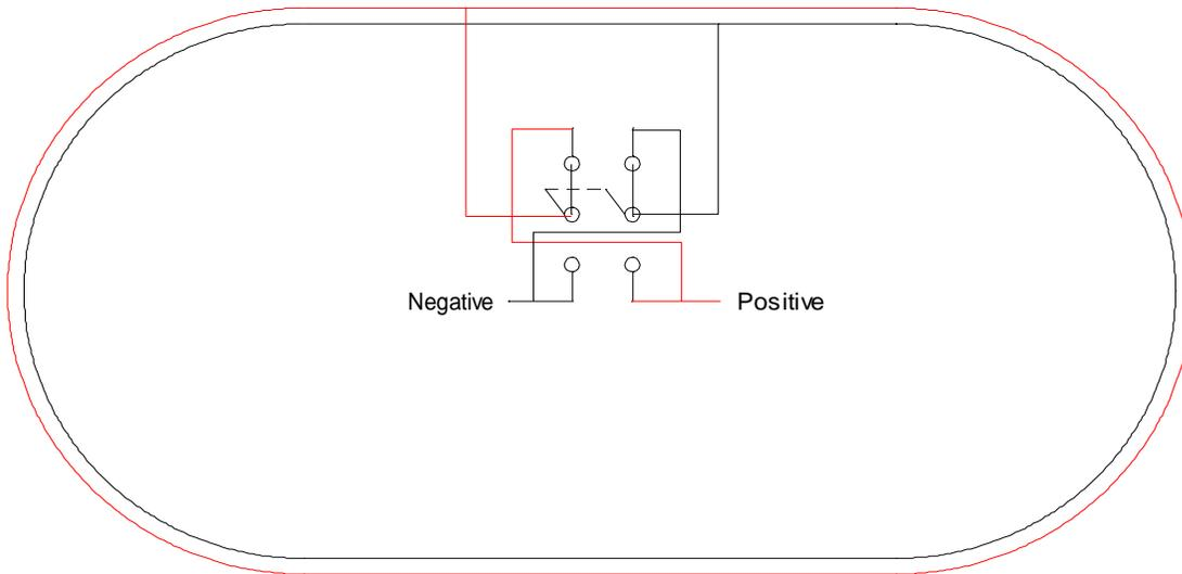
2. When a reverse loop is added to the track plan, two direction switches are needed. They must be wired so they control the polarity independently of each other. Below, the drawing shows the loop and the polarity of the rails. The switch on the left controls the direction inside of the loop and the one on the right controls the train direction outside the loop. Note that with the polarity as shown the train may enter the top of the loop but will short upon reaching the gap near the turnout.
