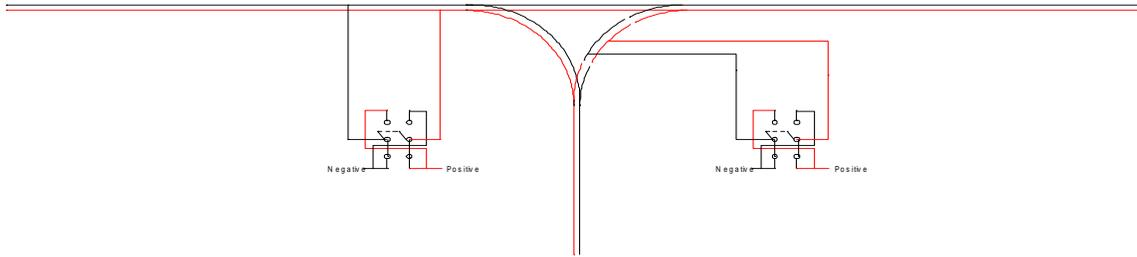
7. Another way of wiring a wye is to have the entire leg as an isolated section. Below, the train can enter the wye leg as before. The length of train is limited only by the length of the wye leg. This is the scheme used on Bremerton Northern Model Railroad's new Kitsap Western Railroad.
