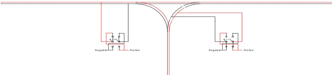
6. While the train is in the isolated section, the main polarity switch is thrown to change the polarity of the mainline. Again, the length of the train is limited to the length of the isolated section (about 36" for 24" radius curve). After the train enters the right hand leg of the wye and stopped, the left direction switch is thrown and the train is turned around, ready to go out.
