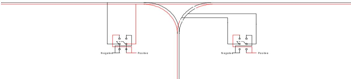
5. After the train is in the wye leg and stopped, it is reversed and the turnouts are thrown. Now the polarity of the isolated section is important and must agree with the direction of the train. Note that at the upper right hand turnout, the polarity conflicts with the isolated section.
