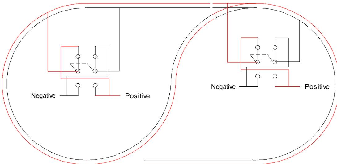
3. While the train is in the loop section, the polarity switch on the right is thrown, thus changing the polarity allowing the train to continue without delay. The schematic shows the gaps near the turnout, but they may be anywhere providing they are at least a train-length apart. The further apart they are, the easier it is to have time to throw the switch while the train is moving. The train need not stop in the loop!
