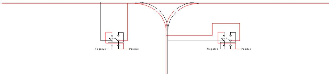
8. After stopping, the turnouts are aligned for the third (right hand) leg, the polarity switch for the wye leg is thrown to change direction of the train, and the reversed train backs onto that leg. All that remains is to stop the train, align the turnouts, change to forward and proceed in the opposite direction.
