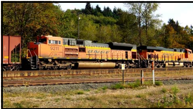
BNSF SD70Ace - 9211 (16-710 2 stroke V16) Location: Chehalis, Time: 4:15 PM Northbound, Unit Tank (DPU)
