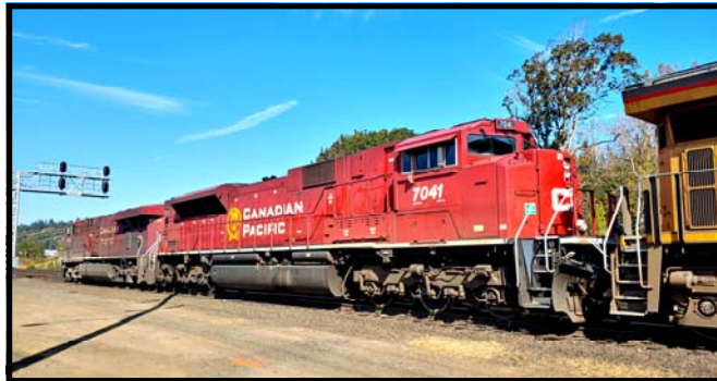
Canadian Pacific SD70ACU-7041 (rebuilt SD90MAC, Progress Rail, 2019-2020, EMD 16-710 G3C) Location: Kalama, Time: 2:06 PM Northbound, Chemical hoppers?
