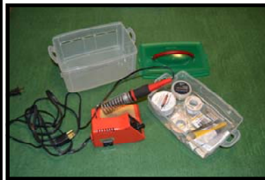
Left: The Soldering Kit with a Weller solder- ing station, assorted tips, flux, a couple rolls of solder, and micro brushes for flux application.
