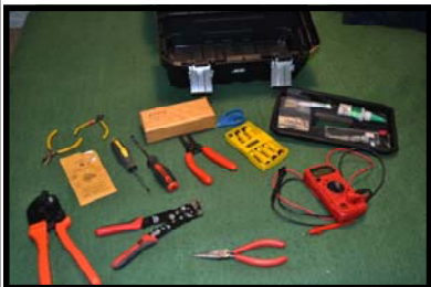
Left: A kit consisting of basic handle tools, an Xacto knife chest, digital multi-meter, NMRA gage and most important a bottle of crazy glue 'un-cure'.
